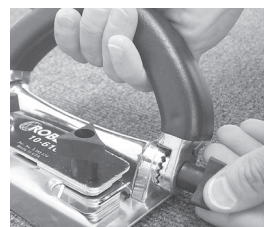
1. Loosen handle knob a full 3-4 turns.
