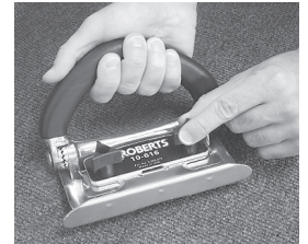
4. Tighten knobs firmly to secure blade holder.
