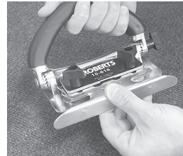
3. Insert the blade holder above the locating plate. Adjust "in and out" dimension for type of carpet being trimmed.
