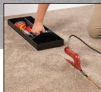
Storage tray with nylon plates acts as a seaming weight
